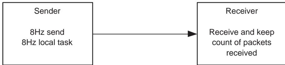
Figure 8: Experimental Setup for Packet Send Throughput
