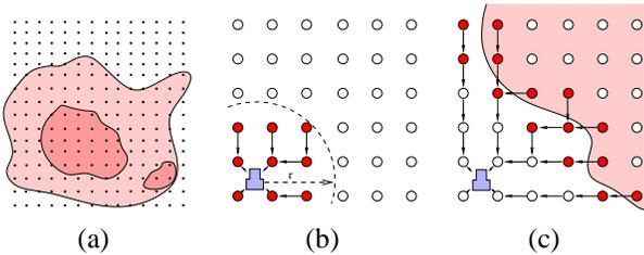
**Fig. 2.** Our sensor network query strategies. (a) Sensor network with different danger levels (darker regions). (b) Spatiotemporal query gets response from the nodes in the vicinity. (c) Border-response query returns the answer from the nodes in the border of danger. Red (darker) circles denote the motes that generate data messages.
