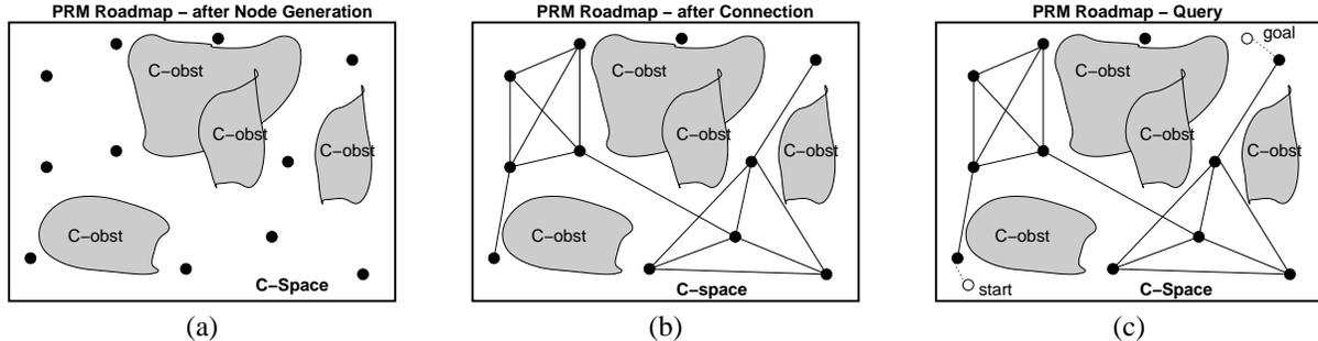
**Fig. 3.** A PRM roadmap in C-space. (a) After node generation, (b) after the connection phase, and (c) using it to solve a query.
