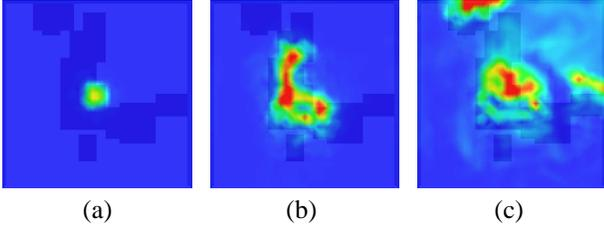
**Fig. 4.** Example simulated sensor readings by our sensor network simulator for a spreading fire. The light regions are high temperature areas.
