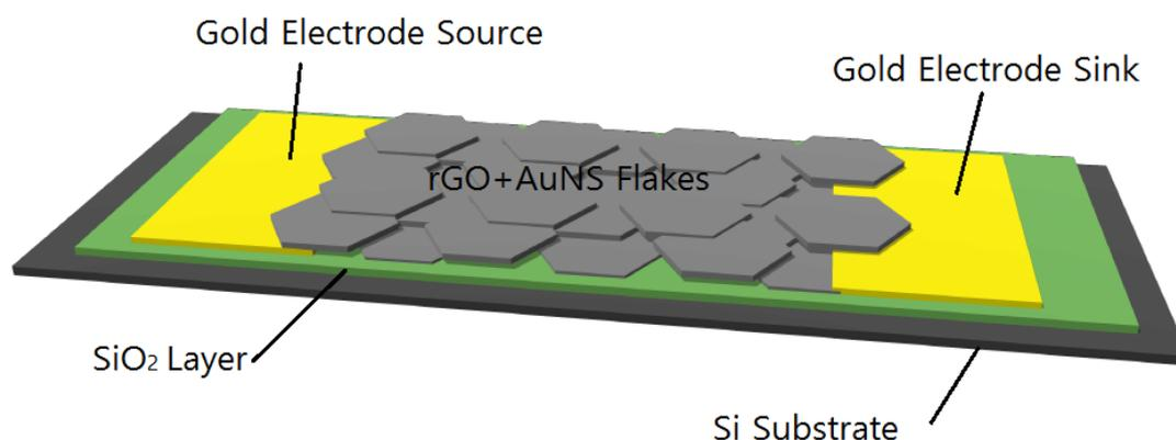
**Figure. 1 Schematic of the electrode.**
