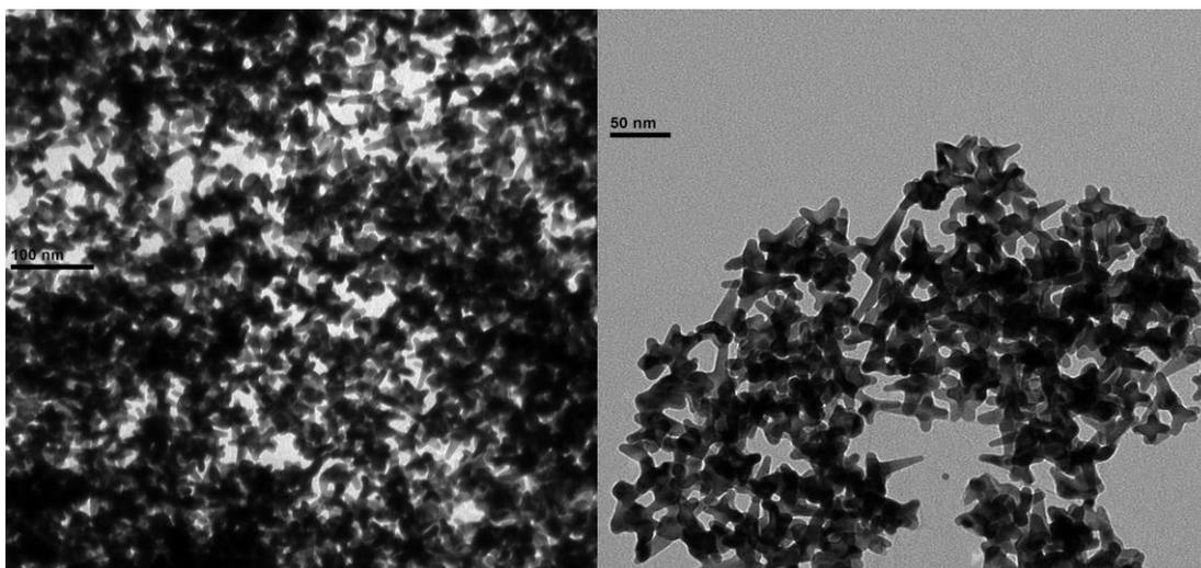
**Figure. 2 AuNS grown on Graphene Oxide layers (TEM)**
