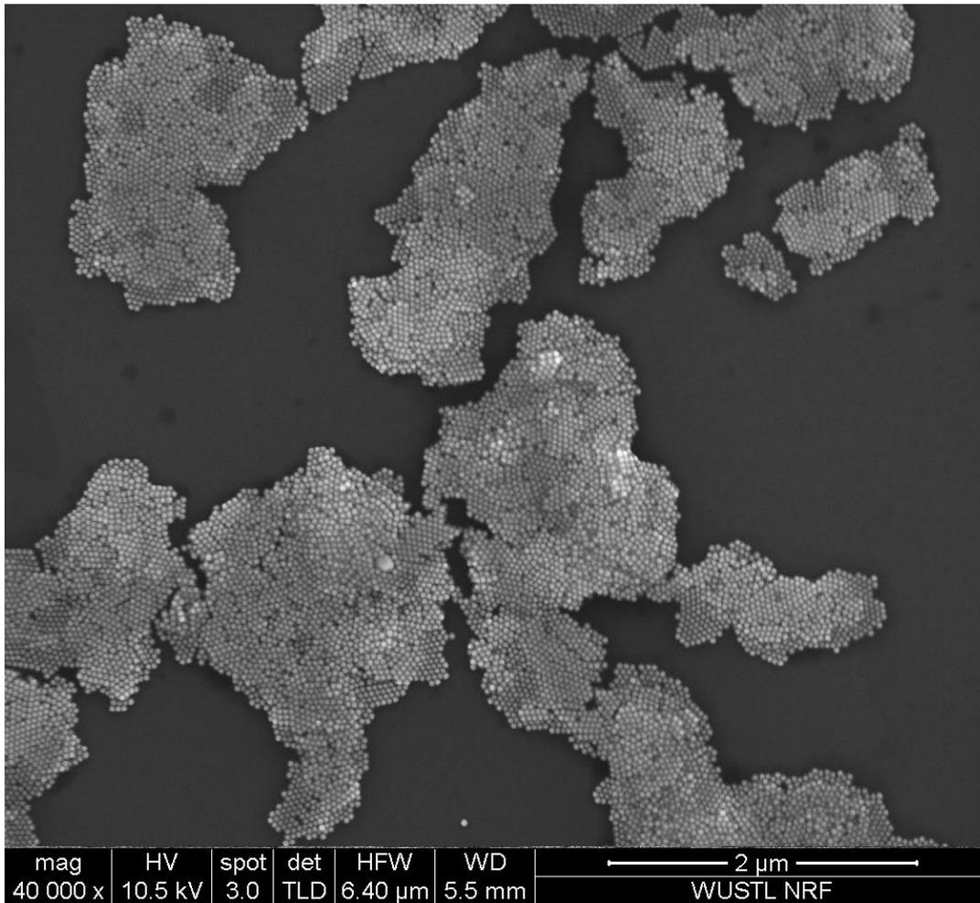
Figure. 10 Gold nanoparticle multilayers from interfacial transfer
