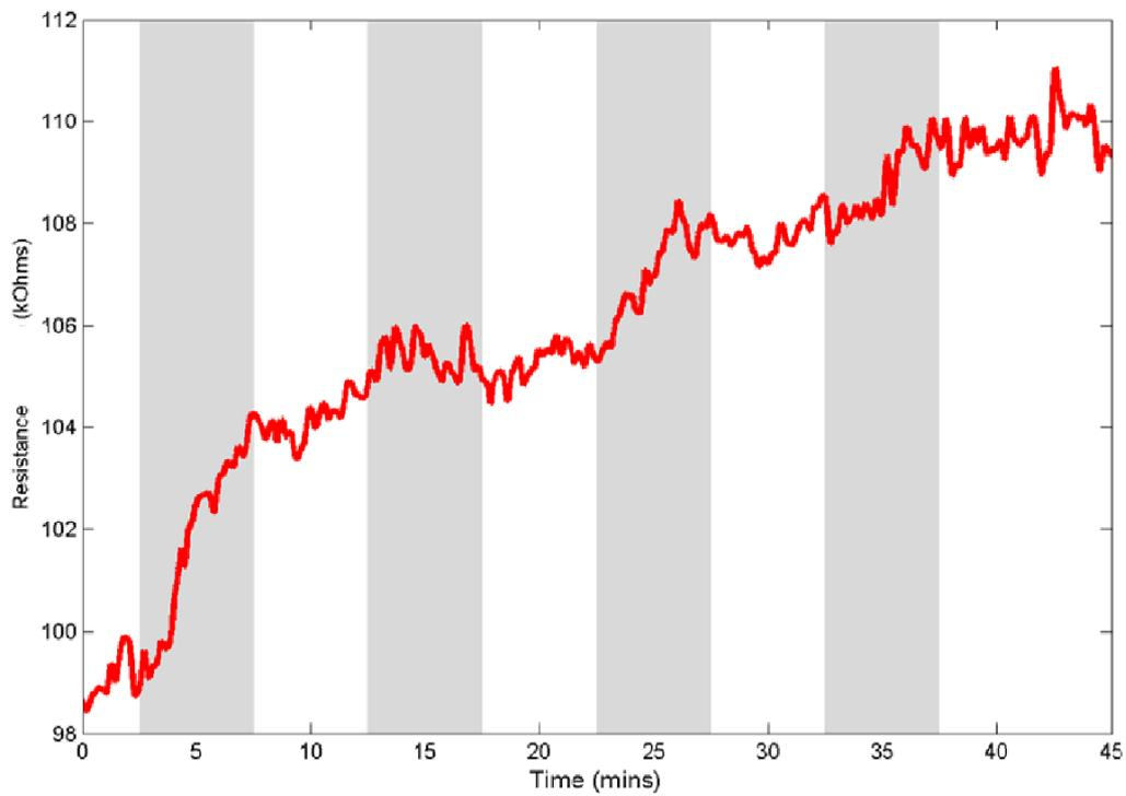
Figure. 4 Resistance change vs. Time under Hexane pulse
