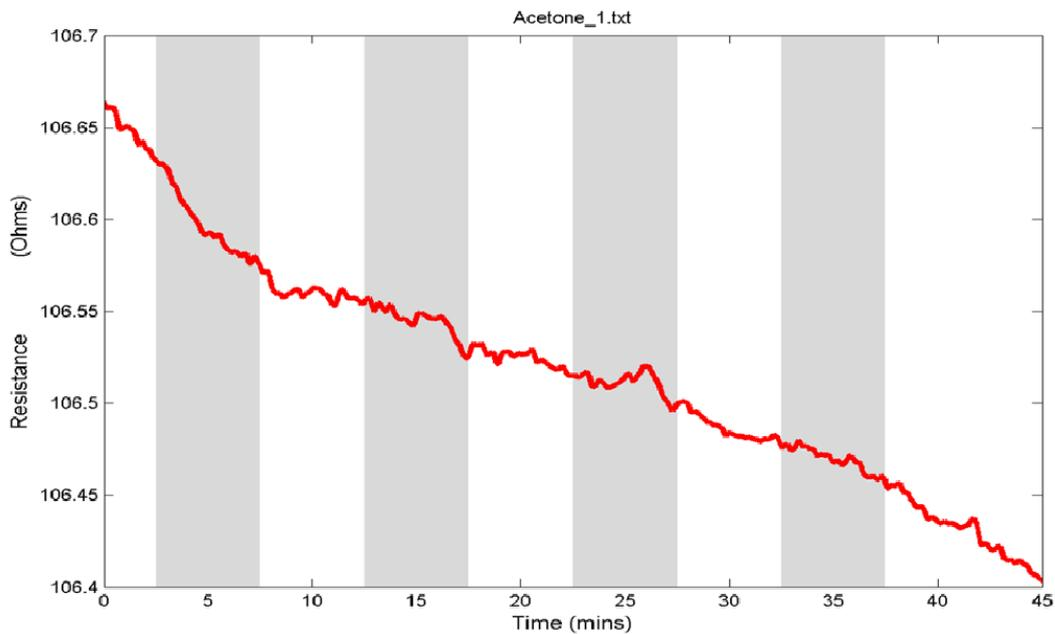
**Figure. 6 Resistance change vs. Time under Acetone pulse**
