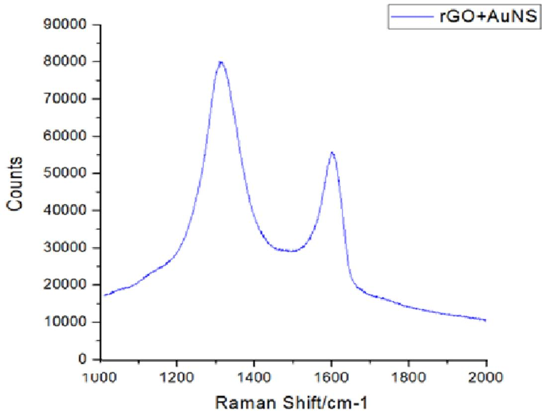
**Figure. 3 Raman spectrum of the GO-AuNS hybrid film deposited on the gold electrode**
