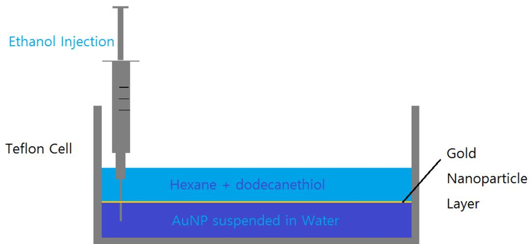
Figure. 9 Schematic of interfacial transfer of gold nanoparticles onto substrates.
