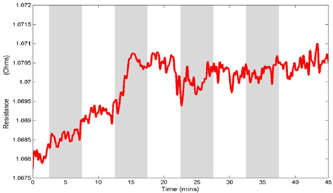
Figure. 5 Resistance change vs. Time under Ethanol pulse
