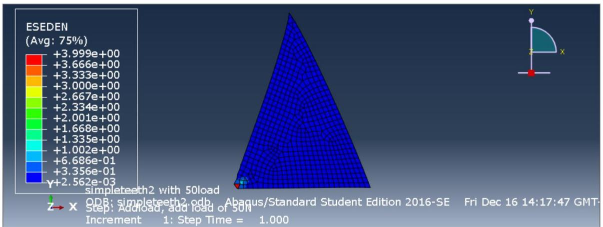
**Figure 3.** Strain energy density. The strain energy density is highest at the singularity associated with the pinned node.
