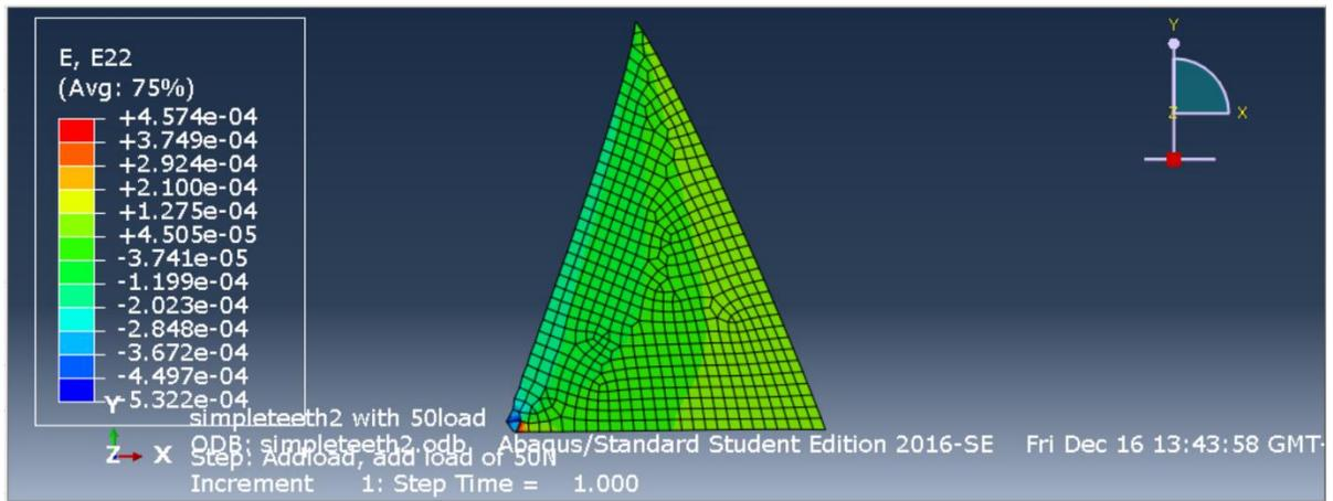
**Figure 2.** Normal engineering strain component in the vertical direction. The strains are generally tensile on the loaded face and compressive on the free face. A strain concentration is evident at the curve of the curved tooth. Both teeth also show the singularity at the point that is fixed.
