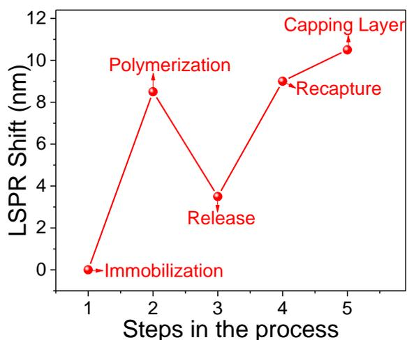
Figure 5 LSPR wavelength of each step in the polymer encapsulation process of the enzyme showing the release and recapture of the enzyme.
