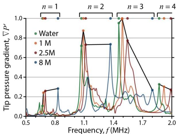
FIG. 3. Simulated resonant frequencies of the 1.2 mm high chamber for various fluid compositions.<sup>[5]</sup>
