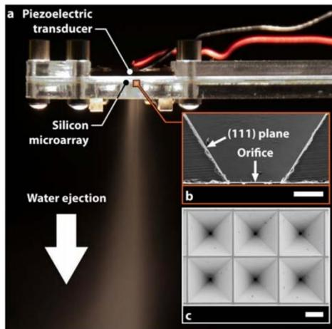
FIG. 2. (a) The uMIST device during operation. (b/c) SEM images of the nozzle geometry.<sup>[7]</sup>
