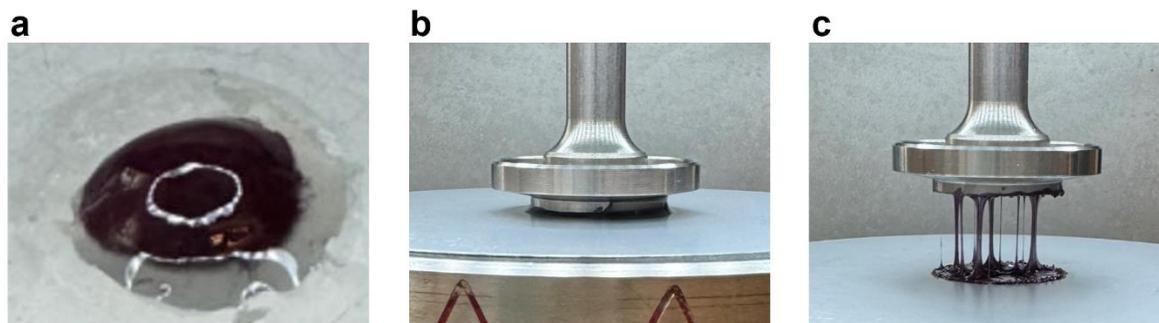
**Figure 2.29.** Pictures of  $C_{2, P1+B3}$  for rheology tests. **a)** as prepared on stage, **b)** before the test covering the gap, **c)** after test.
