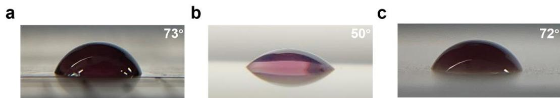
**Figure 2.21.** Representative picture of copolymer  $A_{3,P1}$  on different surfaces: (a) metal, (b) glass, (c) HDPE.
