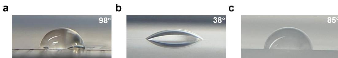
**Figure 2.20.** Representative picture of  $H_2O$  droplets on different surfaces: (a) metal, (b) glass, (c) HDPE.
