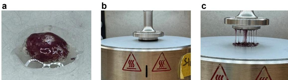
**Figure 2.28.** Pictures of **C<sub>1, P1</sub>+B<sub>3</sub>** for rheology tests. **a)** as prepared on stage, **b)** before the test covering the gap, **c)** after test.
