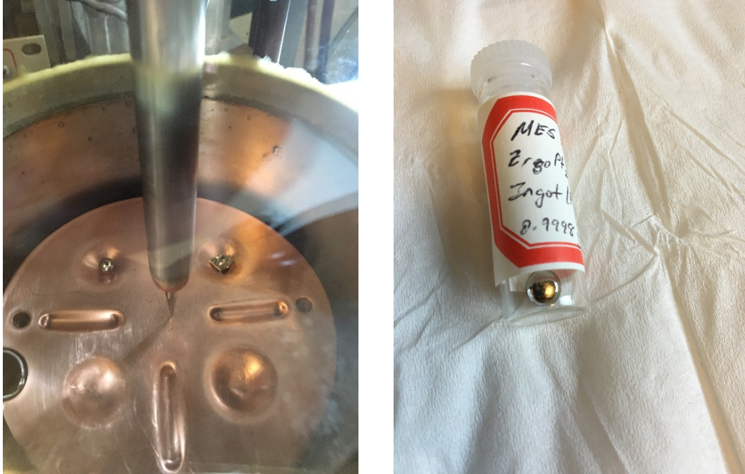
Figure 2.2: (Left) A top-down view of the copper hearth of the arc-melting facility. The vacuum feedthrough and the tungsten tip are positioned in the center of the hearth. At the 10 o'clock position is a \text{Ti}_{50}\text{Zr}_{50} getter, while at the 2 o'clock position is the elemental zirconium crystal bar and platinum wire. (Right) The finished ingot of \text{Zr}_{80}\text{Pt}_{20} after arc melting.
