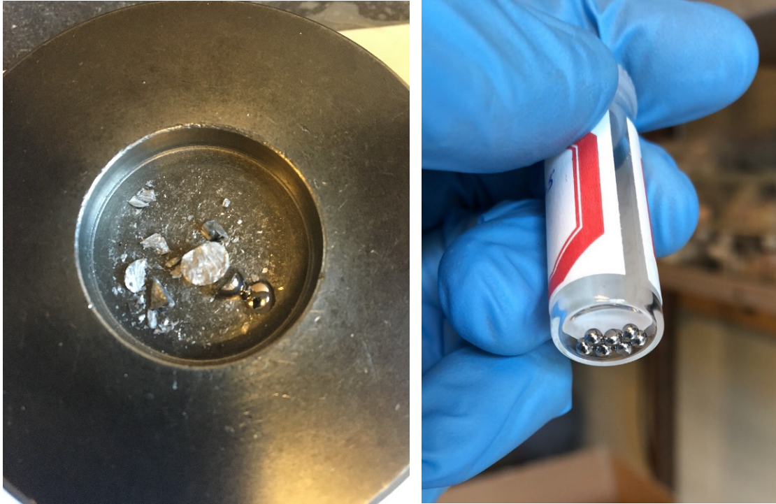
Figure 2.3: (Left) A one-gram ingot crushed into smaller pieces for manufacturing ESL samples. Larger chunks are preferred to minimize the introduction of contamination. (Right) ESL-sized samples after arc-melting them into spheres roughly 2mm in diameter. Seven samples were made from approximately half of the corresponding master ingot. The remaining half of the ingot was kept inside the glovebox under argon for later use.
