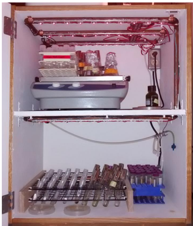
Figure 2.2: Liquid-cooled far-red light chamber interior, showing far-red LEDs, built-in power outlets, shaker, and custom tube rack.
