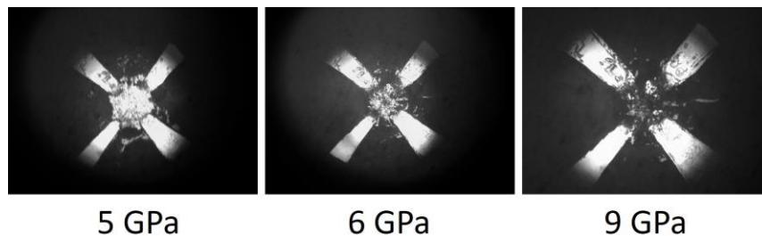
Figure 4.26: Change in reflectivity of Rb where a transition occurs at 5 - 9 GPa pressure. The reflectivity of the four shiny Pt electrical leads to the sample does not change under pressure.
