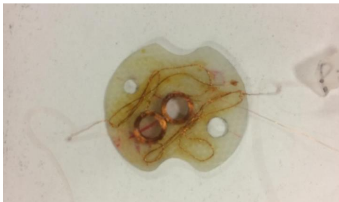
Figure 3.12: Custom coil system for ac susceptibility measurements in the DAC. The central coil is for samples to be measured and the side coil is for a dummy gasket that compensates the magnetic susceptibility signal from the gasket in the central coil.
