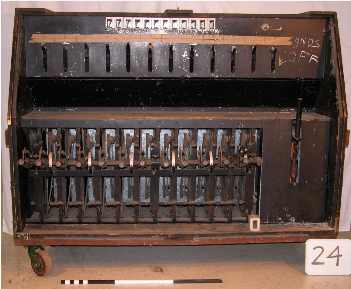
Figure 3.4 An old resistance board, about 4.5 feet tall. For more, see https://blog.etccconnect.com/2017/06/monthly-museum-piano-boards/
