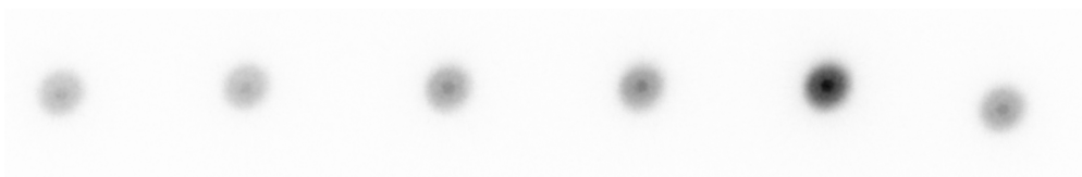
Figure 2.11: Radiographic film showing precision alignment of the sample changer. When the high-intensity central region lies in the center of the diffuse halo, alignment is achieved. All six positions of the sample changer were tested.
