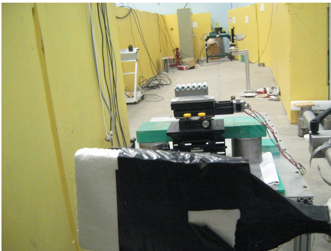
Figure 2.8: Downstream view of monitor detector, sample changer and TOF detectors installed in the 15R beamline.
