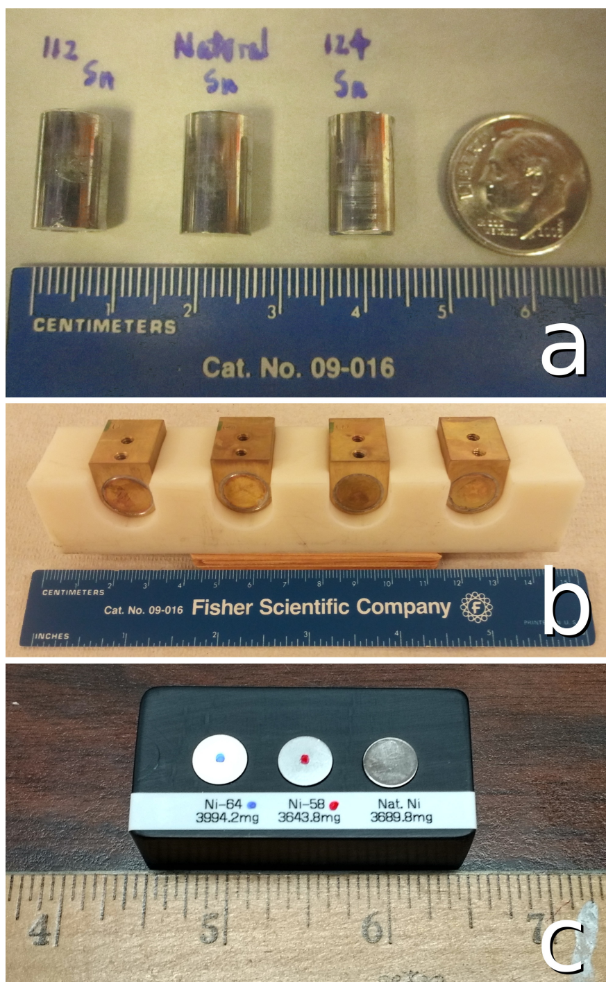
Figure 2.3: ^{112,\text{nat},124}\text{Sn} (section a), \text{H}_2^{\text{nat},18}\text{O} (section b), and ^{58,\text{nat},64}\text{Ni} samples (section c) used for neutron \sigma_{\text{tot}} measurements, with rulers for scale. Brass vessels were used to hold the water samples.
