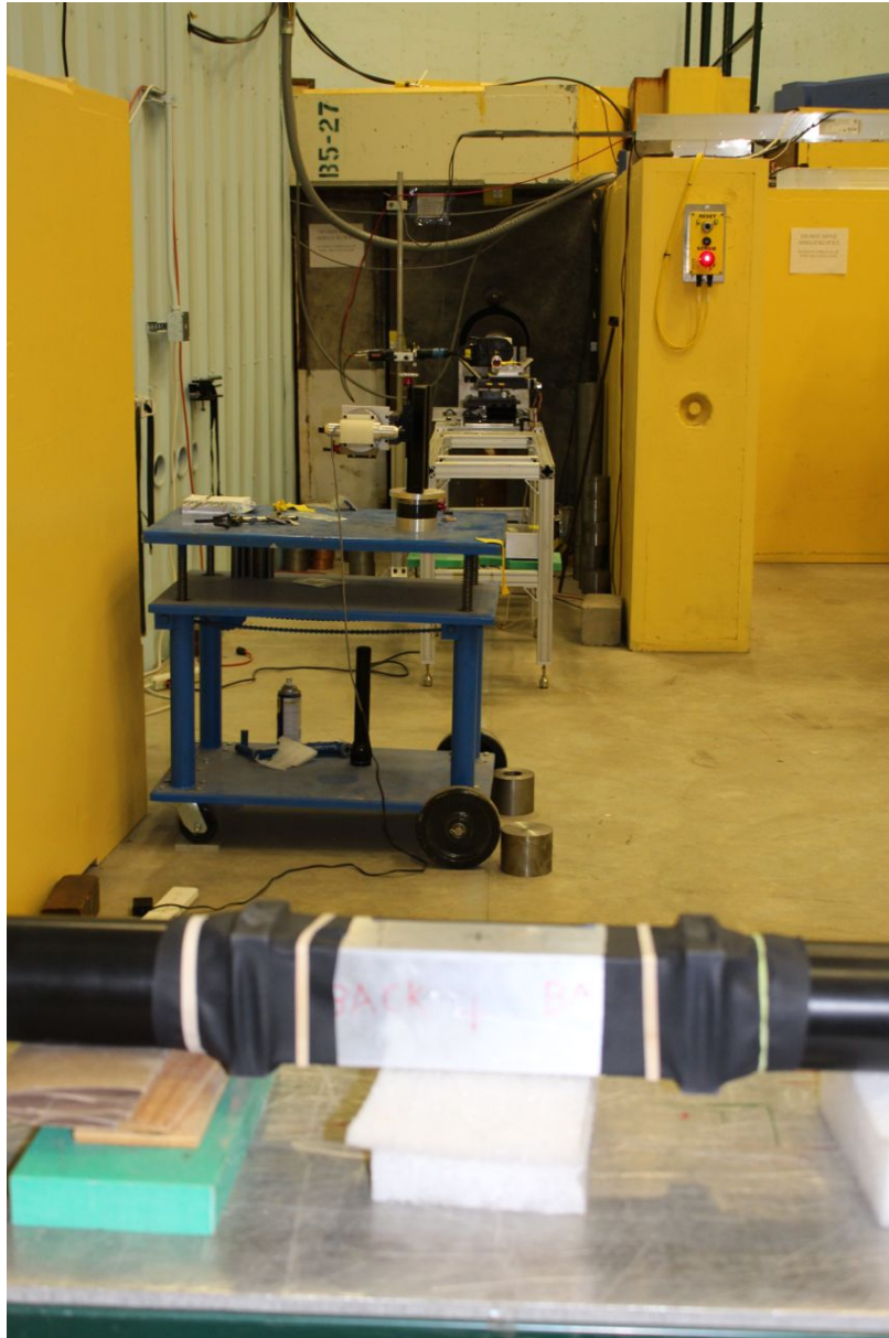
Figure 2.9: Upstream view of \sigma_{\text{tot}} experimental setup in the 15R beamline. In the foreground is the TOF detector (the veto detector is not pictured here). In the background, the sample changer and monitor detector are visible. The blue cart holds the coarse-alignment laser.
