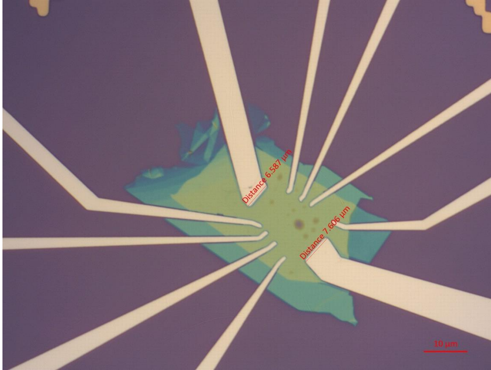
Figure A.12 Photo of device with Al wires (white) made by electron beam evaporation.
