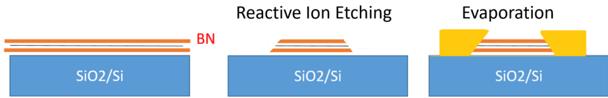
Figure A.15 Schematic process of reactive ion etching and evaporation.
