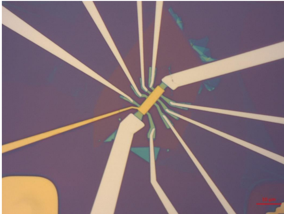
Figure A.16 Pictures of device before and after etching. The Au top gate (yellow) was made by the thermal evaporation.
