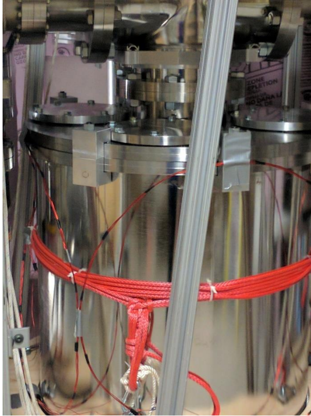
Figure 4.10: The damping coils are mounted on the chamber orthogonal to each other.
