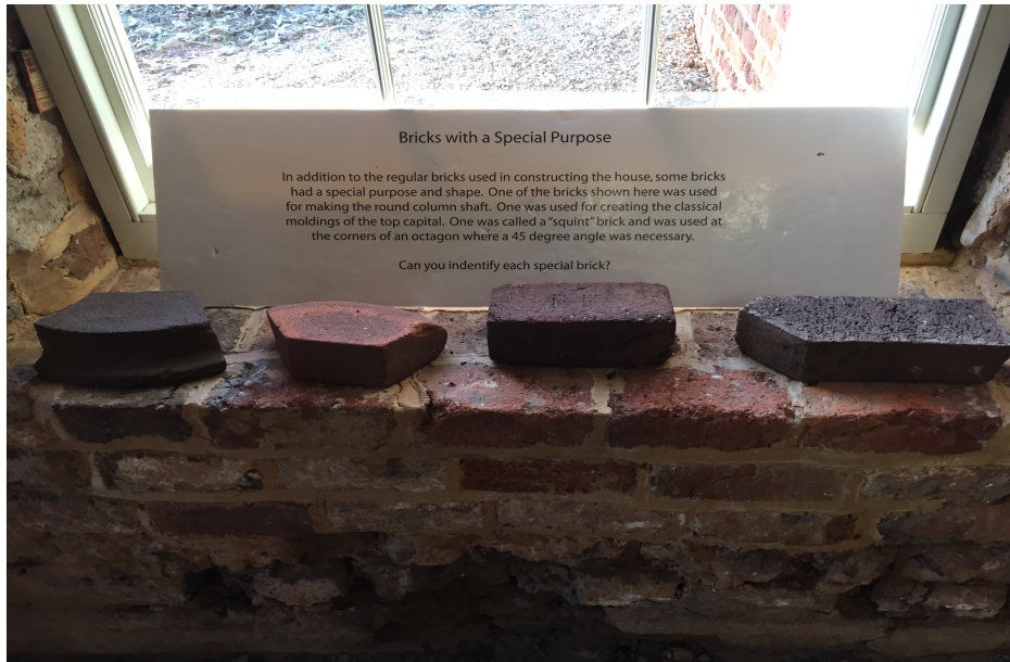
Figure 3. Four of the Six Brick Shapes Used in Poplar Forest Construction (photo taken on 18 November 2018).
