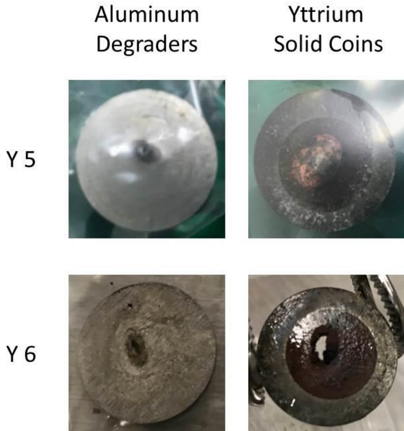
Figure 2-6 Damage to the yttrium coins (Y 5, Y 6) with 2 h irradiation with 12.8 MeV transmitted beam energy (17.8 MeV initial beam energy) and 40 \mu A current.
