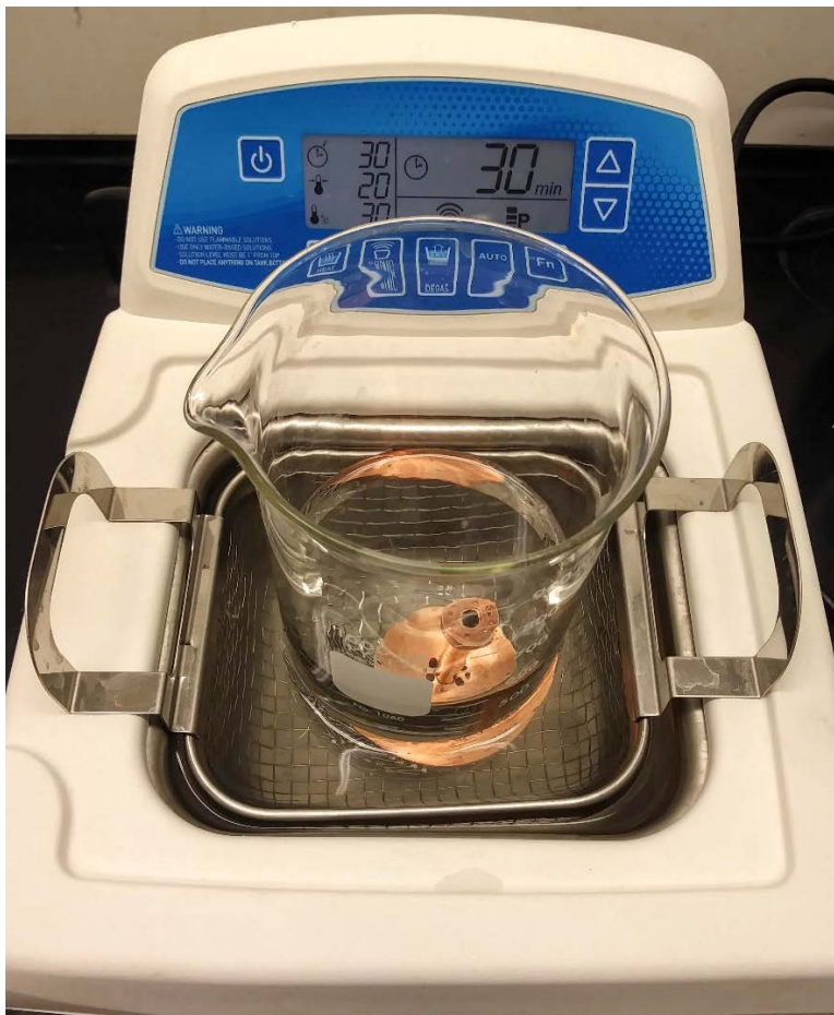
Figure 6.1 Sonicating the internal mode converter taper piece and small screws in ethanol within the sonicator water bath.
