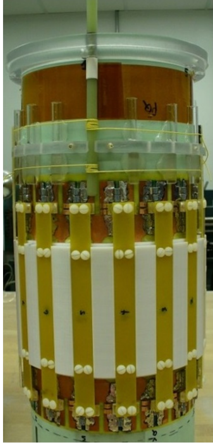
Figure 5.13: A switched-frequency ^1\text{H}/^3\text{He} neonatal-sized birdcage body coil to image lung specimens at both 63.38 MHz (for ^1\text{H} at 1.5T) and 48.65 MHz (for ^3\text{He} at 1.5T).
