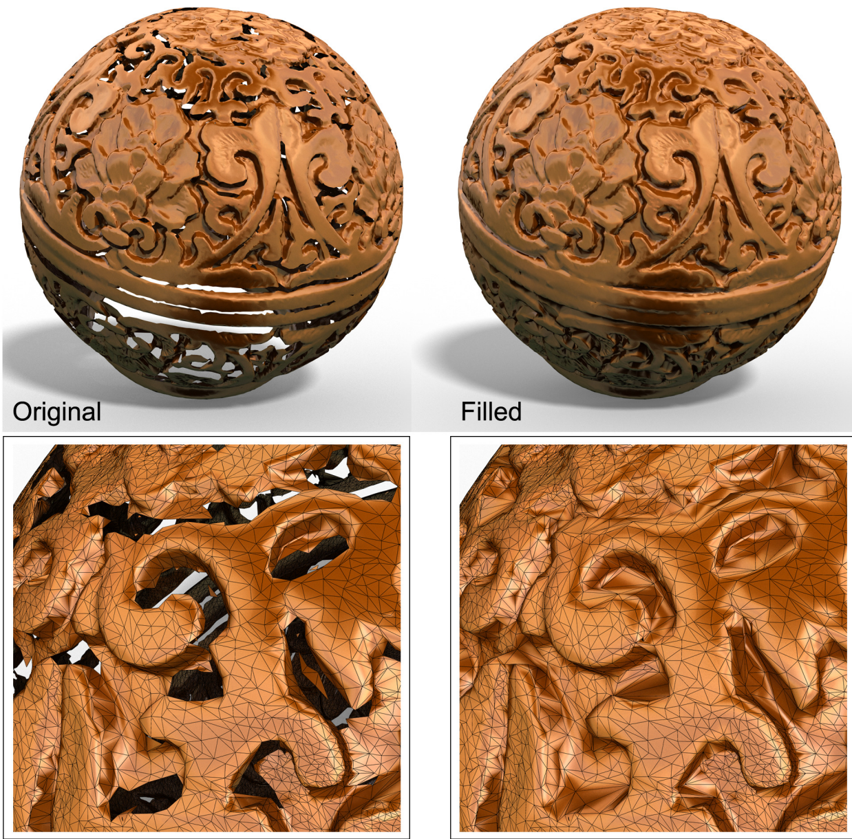
Figure 5.3: Filling a model with numerous holes. Close-ups on a portion of the model are shown at the bottom.
