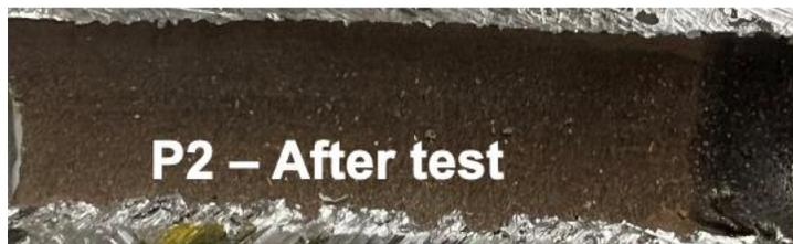
Figure A4.14 Longitudinal cross-sections of control pipes C1', C2', and test pipes P1, P2 after test. The pipes were used for stagnation and free chlorin experiments.
