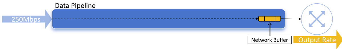
Figure 4.4: Simplified data pipeline with fixed input.
