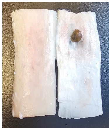
Figure 10. Prepared tendon and bone samples used for adhesion testing with MFP5 adhesive. On the left, the bone sample has been modified to flatten its naturally rounded surface. On the right, the tendon sample has been microtomed into a flat surface, and the brown material is the MFP5 adhesive.
