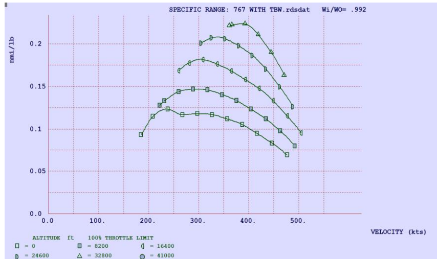
Figure 4.13 B767 TTBW LH2 specific range
