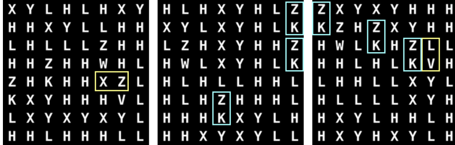
Figure 5.4: Contextual errors were observed in some DDPM-generated realizations from A-SCM. These manifested as incorrect pairings of letters (yellow) or incorrect per-image prevalence of letter-pairs (blue). In the training data, the letter-pairs X-Y, and Z-V were always in order, and the letter-pair Z-K occurred exactly twice in each image.
