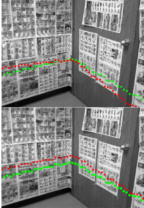
Figure 3. Results of running the auto-calibration for discrete motions. The red circles are the re-projected images of the points measured by the laser range finder using the \Phi and \Delta . Green squares show reprojection using correct (hand calculated) \Phi and \Delta . (Top) After one iteration of algorithm described in Section 4.1.2. (Bottom) After three iterations of alternating refinement of fiducial motion and camera position.
