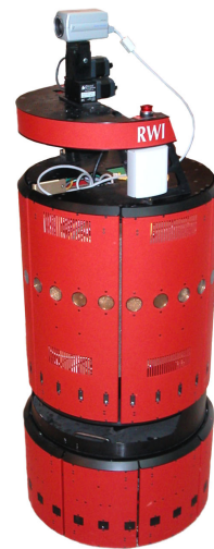
Figure 1. A B21r TM Mobile Robot from iRobot Corporation can be configured to have a video camera (at the top) and a planar laser range finder which measures distances to points lying on a plane about 18 inches off the floor. The goal of this paper is to study auto-calibration methods that find the rotation \Phi and the translation \Delta which transform points in the laser coordinate system to points in the normalized camera coordinate system — by considering data captured simultaneously from both sensors when the robot is in motion.
