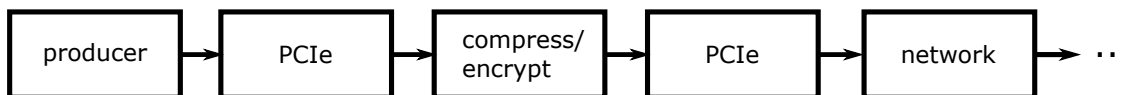
Figure 5.7: Example flow graph for FPGA accelerated compression/encryption using a traditional FPGA interconnection.
