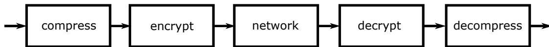
Figure 5.9: Actual flow graph for FPGA accelerated compression/encryption using the bump in the wire configuration.
