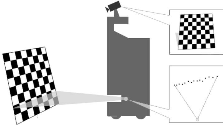
Figure 2: A planar calibration pattern is posed in the both views of the camera and the laser range finder.
