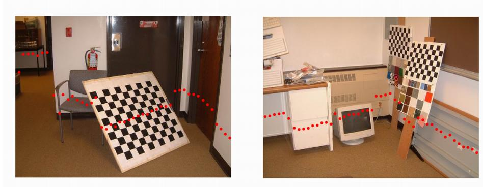
Figure 5: The left figure shows one checkerboard setting captured by the camera, and the red points overlaying on the image are the mapping laser reading with estimated extrinsic parameters  $\Phi$  and  $\Delta$ . The right figure shows one example of laser reading mapped onto the camera image after the extrinsic calibration
