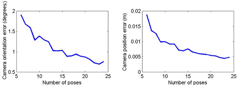
Figure 3: Errors vs. the number of poses of the checkerboard plane
