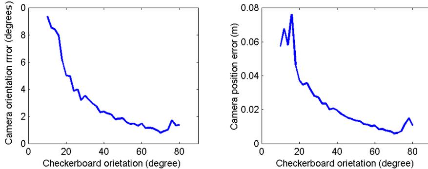
Figure 4: Errors vs. the orientation of the checkerboard plane
