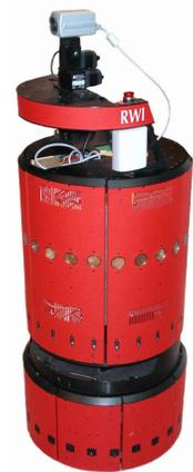
Figure 1: A B21r<sup>TM</sup> Mobile Robot from iRobot Corporation can be configured to have a video camera (at the top) and a planar laser range finder which measures distances to points lying on a plane about 18 inches off the floor. The goal of this paper is to study a calibration method that finds the rotation  $\Phi$  and the translation  $\Delta$  which transform points in the camera coordinate system to points in the laser coordinate system
