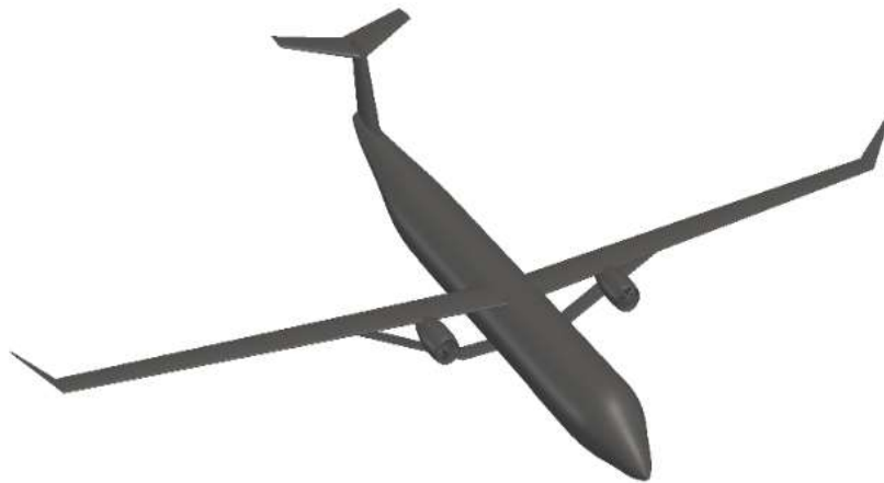
Figure 5.4 Aircraft configuration with a truss braced wing
