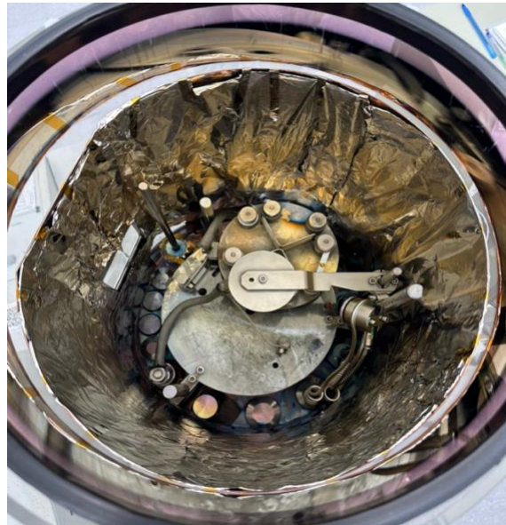
Figure 9: The interior walls of the PVD-Thermal Evaporator.
