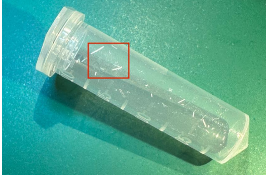
Fig 1: Sample image of Bi 2 SeO 5 used for the device fabrication for this thesis.
