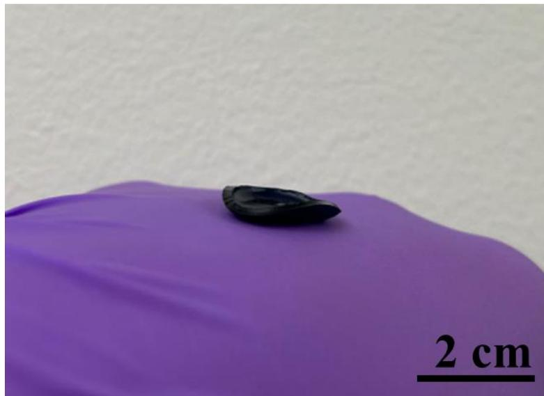
Figure 2.12 Photograph of suction-cup shaped hydrogel epidermal electrode.
