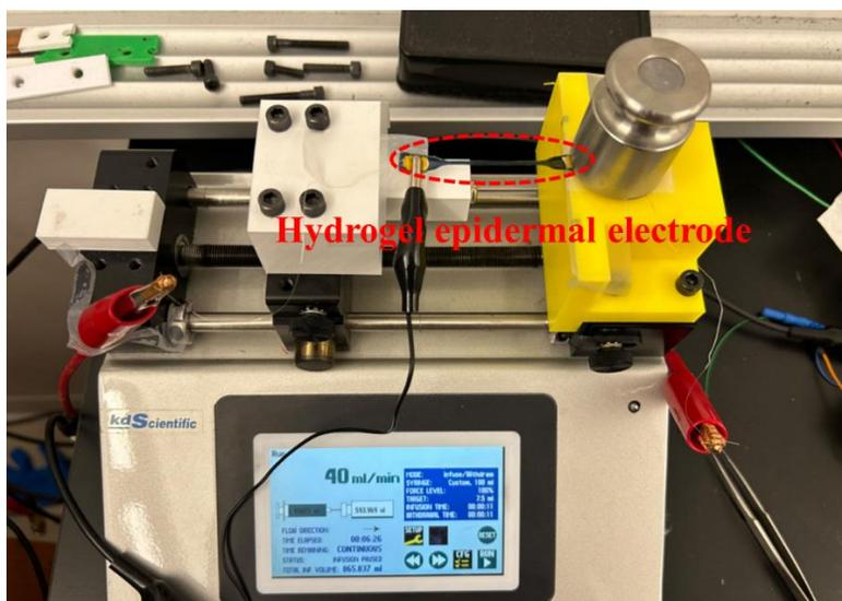
Figure 3.6 Measurement device for tensile resistance change of hydrogel epidermal electrode.
