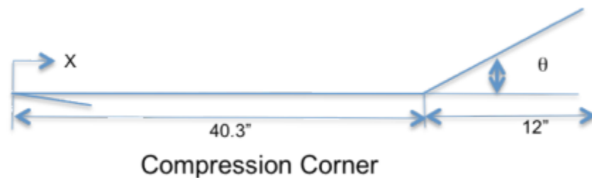
Figure 2.1 Schematic of the compression corner geometry. [11]
