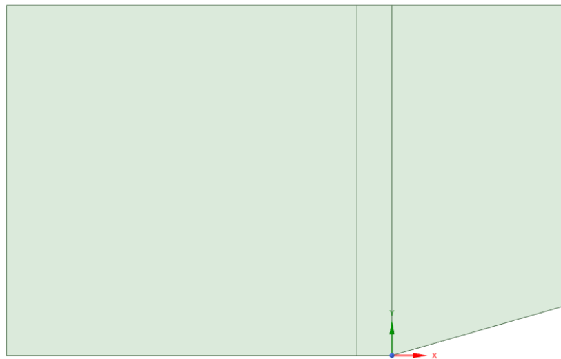
Figure 2.4. Flow domain geometry of the 16-degree Settles' compression corner.
