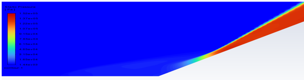
Figure 3.67 Pressure contours and oblique shock for Holden's case at Mach 11.3 for 36-degree corner angles using WA model.
