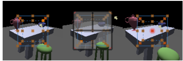
Figure 3: Camera Dolly And Zoom With Focal Planes: A camera dolly and zoom is accomplished by zooming out/in while dollying in/out to keep the size of the cube the same. The depth of the focus point can be changed by sliding a focal plane through the scene.
