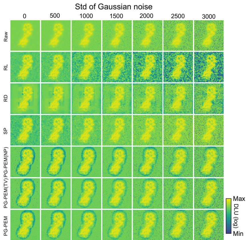
Figure 3.9: Restoration results from different noise levels and methods when \alpha = 20 (log scale). It is easier to compare the denoising ability between different methods using the log-scale images.
