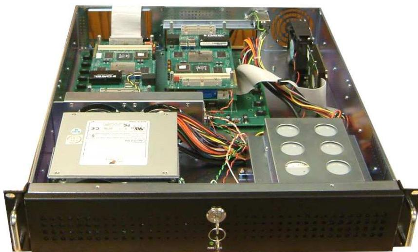
Figure 5.3: FPX-in-a-Box System
