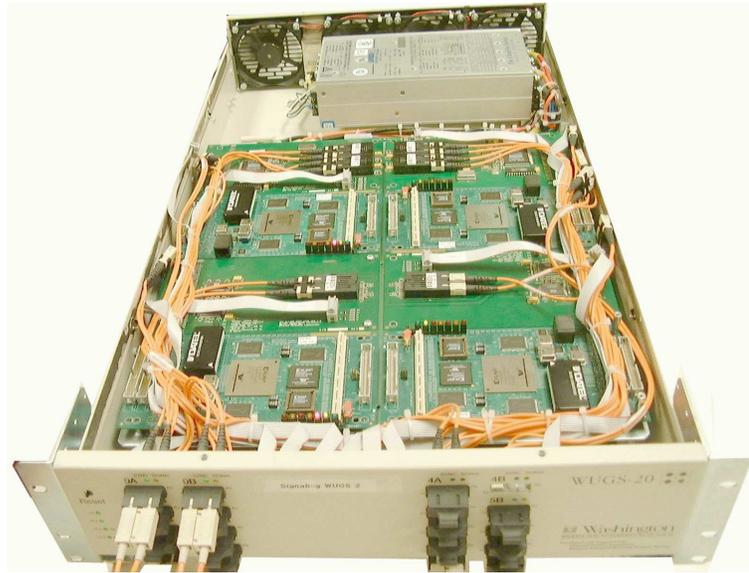
Figure 5.2: Washington University Gigabit Switch Loaded with Four FPX Cards
