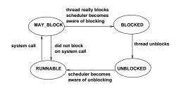
Fig. 4. State Transition for Threads
