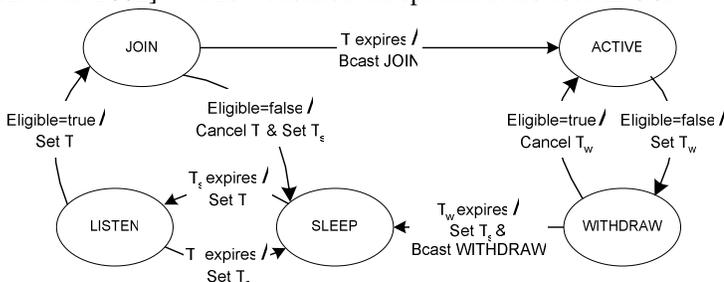
Fig. 10 State diagram of CCP
