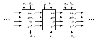
Figure 1: Iterative structure of range check circuit
