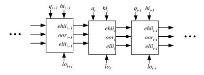
Figure 6: Iterative structure of revised range check circuit
