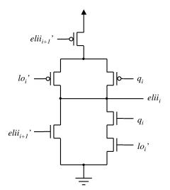
Figure 8: Sub-circuit for *equals-hi-if-in-range* signal
