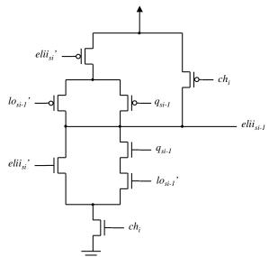
Figure 11: Sub-circuit for equals-hi-if-inrange signal for input to stage si - 1
