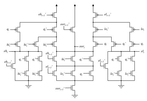
Figure 5: Range-check sub-circuit using three inter-stage signals
