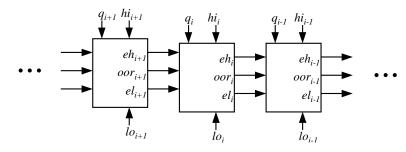
Figure 4: Iterative structure of range check circuit
