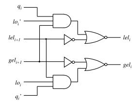
Figure 2: Range-check sub-circuit for upper bound comparison
