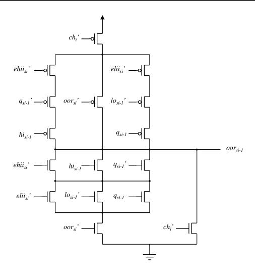
Figure 10: Sub-circuit for *out-of-range* signal for input to stage si - 1
