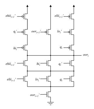
Figure 7: Sub-circuit for *out-of-range* signal
