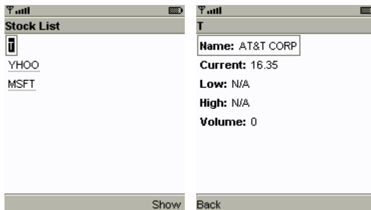
Fig. 5. Left: the client stock ticker on a mobile phone emulator, displaying a list of discovered stock monitors. Right: the client displaying the value of a selected stock.
