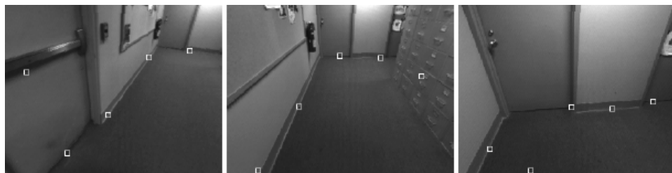
Figure 2.1: Environment and detected features from Martin [23]. The white boxes indicate the evolved program’s predictions for the lowest non-floor pixel in the column.
