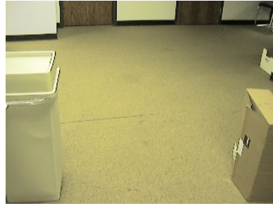
Figure 4.1: Two obstacles at the left and right edges of the image are used to eliminate laser data that is outside the robot's field of view.
