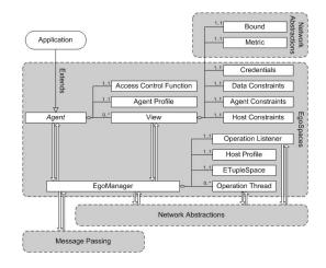
Fig. 11. Internal class diagram of EgoSpaces
