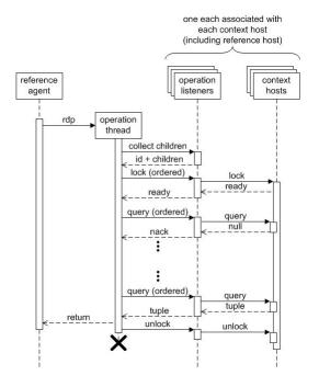
Fig. 13. Sequence diagram of a rdp
