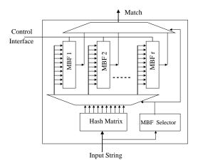
Figure 7. A large Bloom filter (LBF) constructed by using multiple mini-Bloom filters (MBF). The signatures are distributed uniformly randomly among all the MBFs. With r MBFs,  $r\times 1419$  strings can be stored in this LBF
