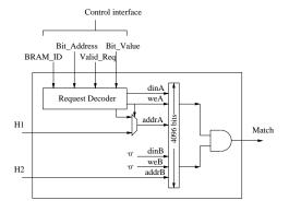
Figure 5. A Partial Bloom filter (PBF) with k=2 hash functions and m=4096 bits. This filter can accommodate n=1419 strings with false positive probability  $(1/2)^2$ .
