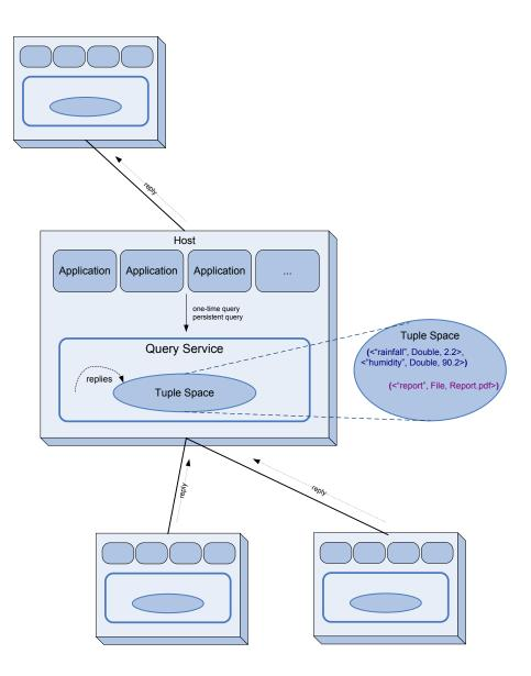
Figure 1: Each host in the ad hoc network is equipped with our query service, which uses tuples for data representation and tuple spaces for storage.
