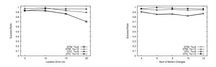
Fig. 16. Success ratios with location errors. The query period is 0.5s, the user speed is  $3 \sim 5m/s$ , and the sleep period is 15s.
