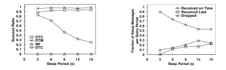
Fig. 8. Success ratios of DTC, DTM and OTC. The user speed is  $3 \sim 5m/s$ . The query period is 0.5s.
