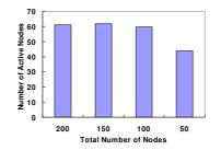
Fig. 14. Success ratio for different node densities. The query period is 0.5s, the user speed is  $3 \sim 5m/s$ , and the sleep period is 9s.
