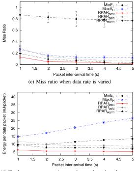
(d) Total energy consumption per data packet when data rate is varied
