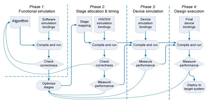
Figure 1: The Auto-Pipe design flow.
