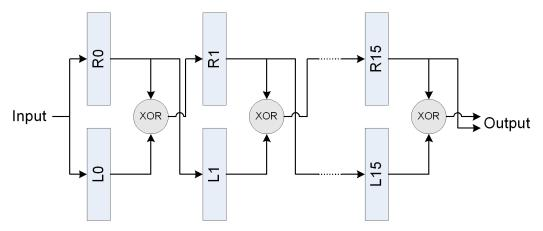
Figure 2: Triple-DES algorithm block diagram. L blocks  $\equiv$  left 32 bits; R blocks  $\equiv$  right 32 bits.
