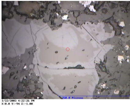
Figure 9. Reflected light image of the location of traverse 2 on the Lunar Crater phenocryst with a stack of spectra showing spectral changes across the alteration front. The direction of the traverse was normal to the alteration front at the location of the spot shown. Distances are reported according to the spacing of the Raman spectra ( 2 \mu\text{m} steps). The secondary phases present in the alteration products include goethite and a 'polymerized' phase (see text).
