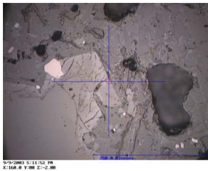
Figure 13. Reflected light image of the location of traverse 5 on Mauna Kea sample 16J-30 with a stack of spectra showing spectral changes across the front. The traverse was oriented along the x-axis of the cross-hairs as shown. Distances are reported according to the spacing of the Raman spectra (2 \mu\text{m} steps). Secondary phases include a polymerized silicate and traces of an iron oxide, inferred to be maghemite from the microprobe data.
