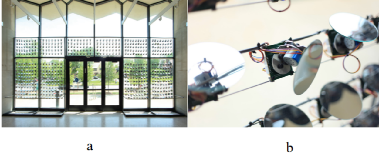
Figure 1.2: (a) Image of the entire catoptric surface system. (b) A part of mirrors in the system with a close-up image of an individual module [1].
