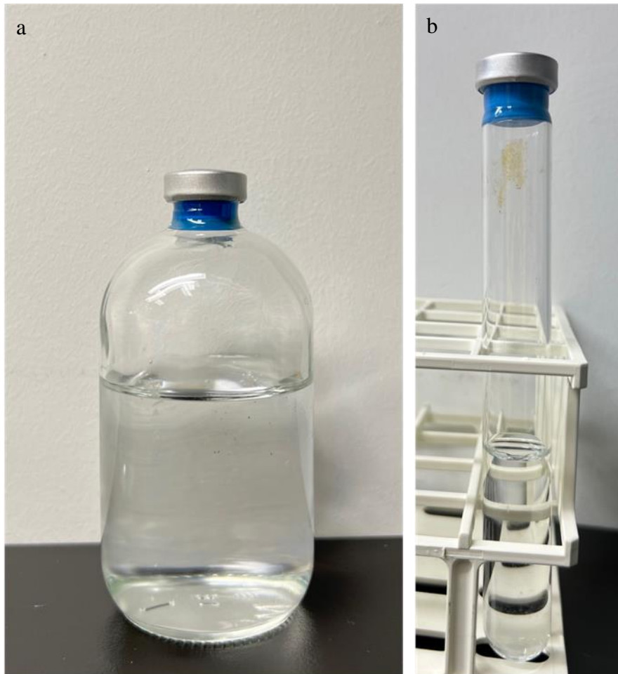
Figure 2. 1 Anaerobic pressure bottle and tube. (a) The anaerobic pressure bottle, which consists of three parts, the glass bottle, the blue rubber plug and the aluminum ring. The aluminum ring was clamped to ensure the plug stayed on the bottle during autoclave. (b) The anaerobic pressure tube.
