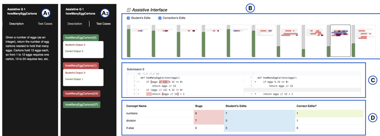
Figure 4.1 The Assistive Interface: (A1) problem description; (A2) test cases for this problem; (B) Submission History Snapshots; (C) the selected submission and its closest correction; (D) a concept table that maps required concepts with bugs and student's edits
