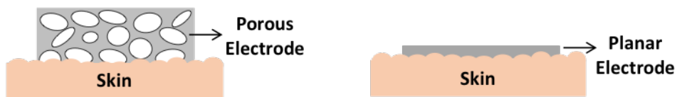
Figure 4.5: Schematics illustrating the difference in skin-electrode contact area between the porous electrode and planar electrode when no conductive hydrogel is used. The porous electrode has a typical pore size in the range of 300 – 500 \mu\text{m} and a porosity of 0.6192. When no conductive gel is used, the measured electrode-skin contact impedance is 247 \text{k}\Omega for the planar electrode, which is slightly lower than the 277 \text{k}\Omega measured from the porous electrode of the same size. The difference can be attributed to the fact that some micropores in the sponge electrode are only partially in contact with the skin surface, resulting in a slightly smaller skin-electrode contact area compared to the planar electrode.
